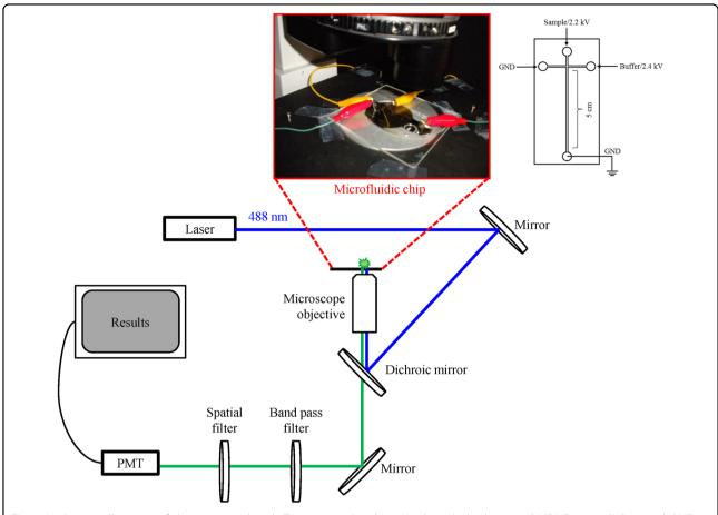
Fig. 4 A schematic illustration of chip geometry (simple-T 5 cm microchip design) with applied voltages and ME-LIF setup. GND ground, PMT photomultiplier tubes
