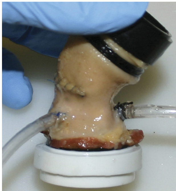
Fig 2. Human homograft roots were implanted in the pulse duplicator to study transcatheter aortic valve implantation.
